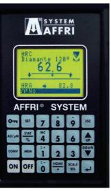
high contrast to obtain clear, rapid and accurate readings. Icons facilitate the operator in identifying software functions. - Signal for test cycle end that facilitate the operator - The operator can automatically select test load and measure scale only though a button - Simultaneous conversion different scales (Rockwell, Brinell, Vickers and in N mm2 resistance)
