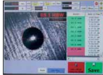
Automatic Brinell / Vickers and Auto Focus
