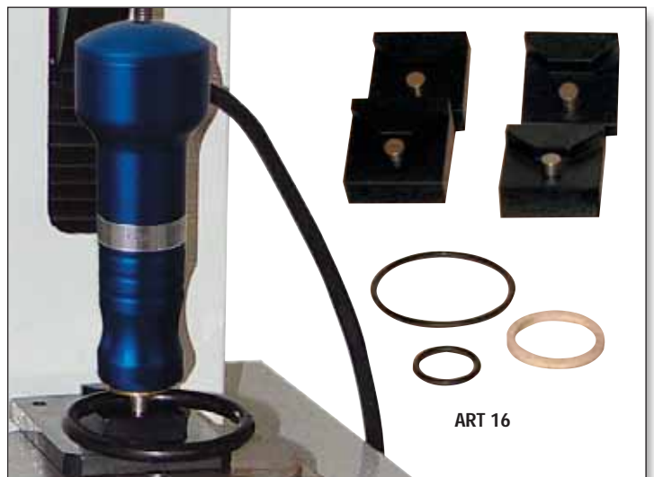
ART 16 Set of clamping holders for bench connection in compliance with ASTM 1414 for precise test O-Ring (section \varnothing 1,72 - 2,54 - 3,43 - 5,21 - 6,83 mm)
