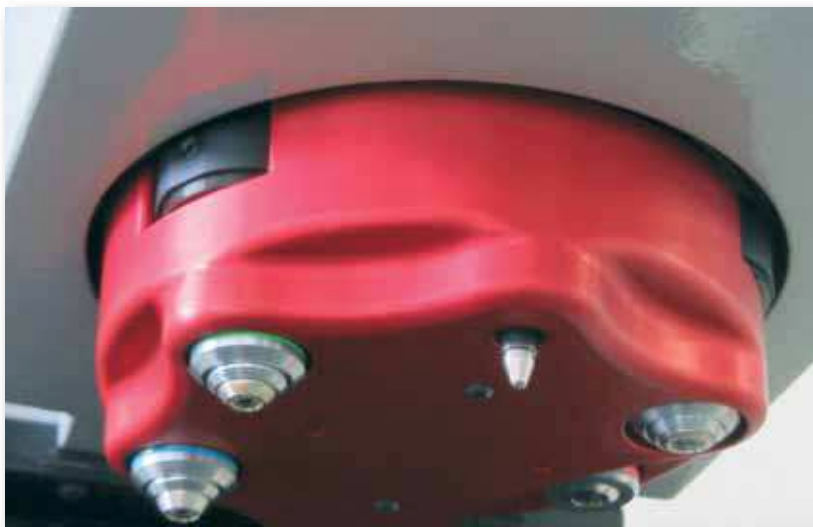
New rotary selector. All objectives and indenters can be installed and automatically combined on rotary turret. It performs a quick test cycle that optimizes the magnification.
